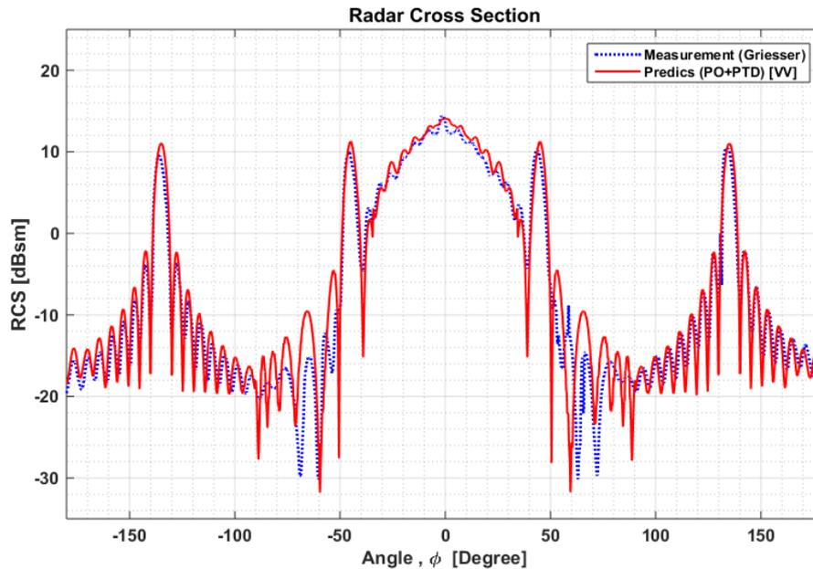
**Figure 5.** Angular RCS results comparison with respect to the measurement of [2] and PREDICS's simulation [PO+SBR+PTD solver]
