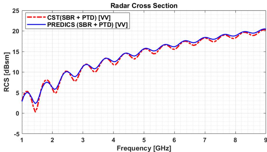
**Figure 7.** Comparison of spectral RCS results between PREDICS [SBR+PTD] solver, and CST asymptotic [SBR+PTD] solver for the TCR object
