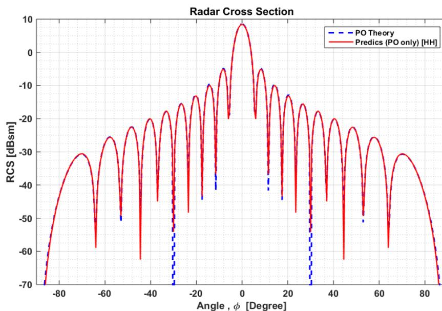
**Figure 2.** RCS results by PREDICS simulation [PO solver] compared to PO theory
