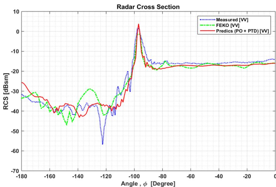
**Figure 9.** Angular RCS PREDICS result [PO+PTD solver] in comparison with respect to measurement of [4] and FEKO simulation
