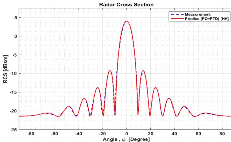
**Figure 3.** RCS results by PREDICS simulation [PO+PTD solver] compared to the measurement RCS provided in [2]
