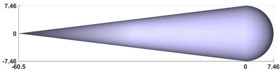
**Figure 8.** The cone-sphere geometry [67.96 cm x 14.92 cm x 14.92 cm]
